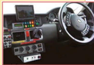
Dashboard Mounted VDS (Fuel Delivery Vehicle)
